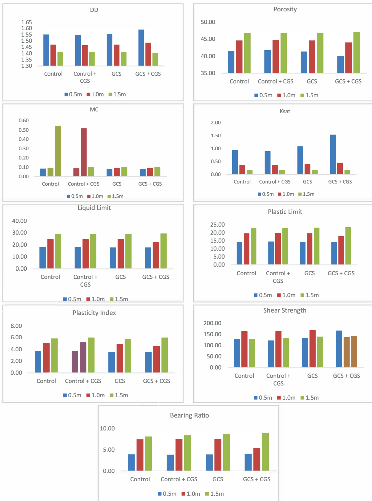
Fig. 2b. Soil hydro-geotechnical properties as affected by amended and un-amended control and greywater-polluted soils
