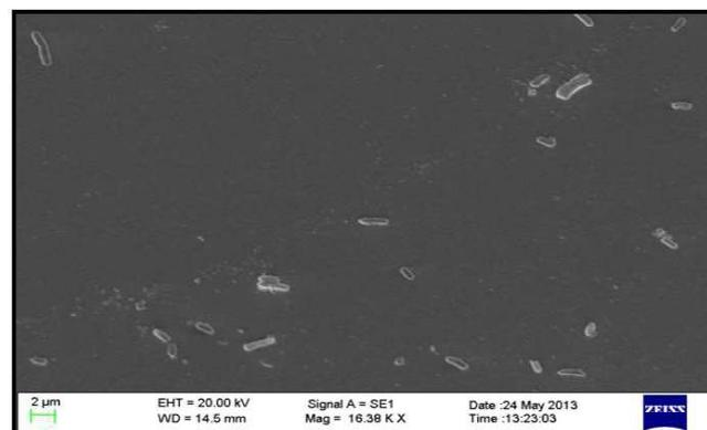
**Fig.4. Scanning electron microscope micrograph of biofilms of Jal1, grown on glass substratum at 16.38KX magnification**
