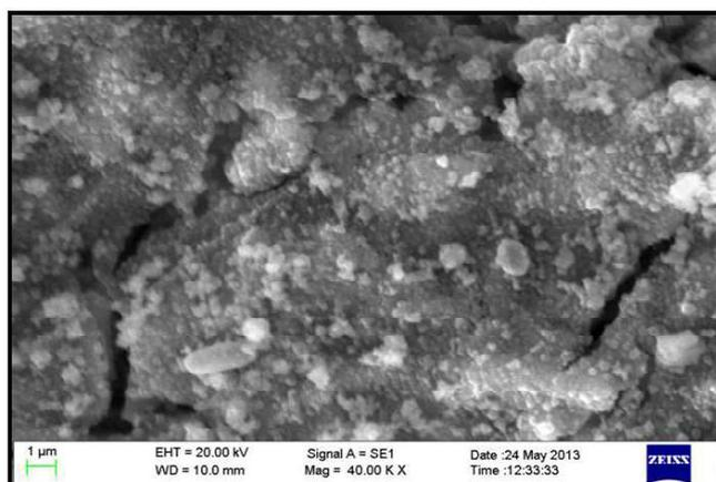
**Fig.1. Scanning electron microscope micrograph of biofilms of the reference *Cronobacter sakazakii* MTCC-2958 grown on steel substratum at 40KX magnification**
