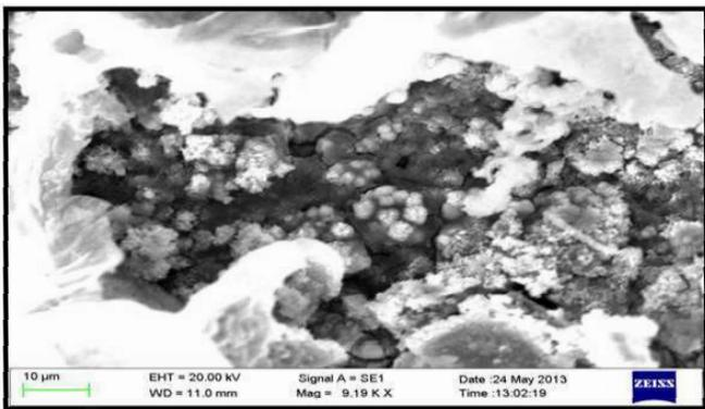
**Fig.6. Scanning electron microscope micrograph biofilms of Jal1, grown on aluminium substratum at 9.19KX magnification**
