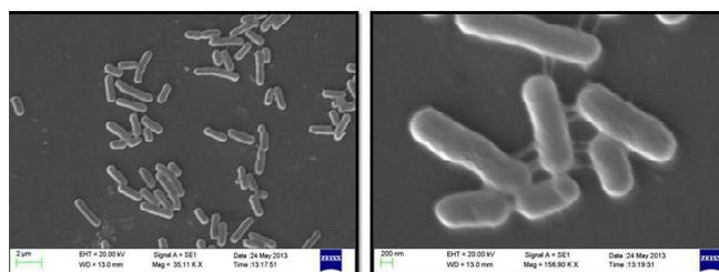
**Fig.3. Scanning electron microscope micrograph of the reference *Cronobacter sakazakii* MTCC-2958 grown on steel substratum (a) at 35.11KX magnification (b) at 156.90KX magnification showing adhesion threads**
