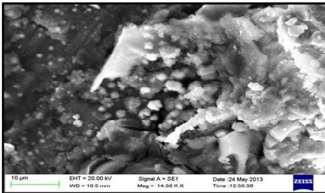
**Fig.5. Scanning electron microscope micrograph of biofilms of the reference *Cronobacter sakazakii* (MTCC-2958) grown on aluminium substratum at 4.36KX magnification**
