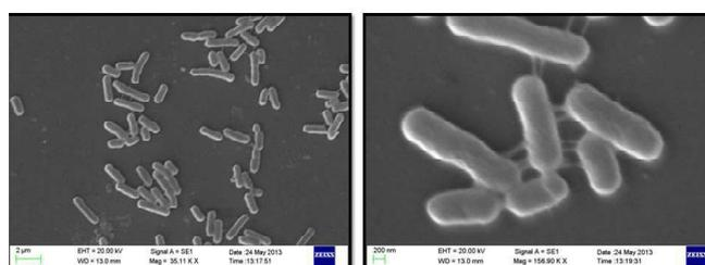
**Fig.3. Scanning electron microscope micrograph of the reference *Cronobacter sakazakii* MTCC-2958 grown on steel substratum (a) at 35.11KX magnification (b) at 156.90KX magnification showing adhesion threads**
