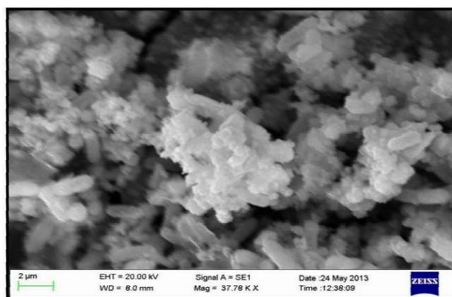
**Fig.2. Scanning electron microscope of biofilms of Jal1, grown on steel substratum at 37.78KX magnification**
